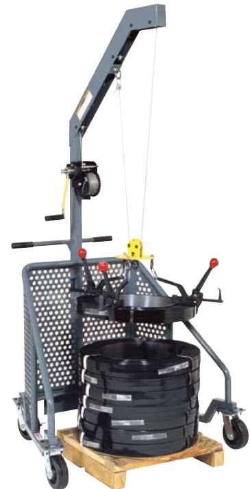
Coil Lifter Capable of lifting up to 125 lb. strap coils, the standard coil lifter is designed for easy dispenser loading, both vertically and horizontally. Accommodates both mill and ribbon wound steel strap coils as well as standard plastic coils. Available in a stationary (Part No. 425650) or portable model (Part No. 424700).
