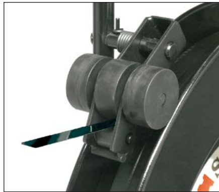
Straproller Feature Prevents strap spillage and tangling.
